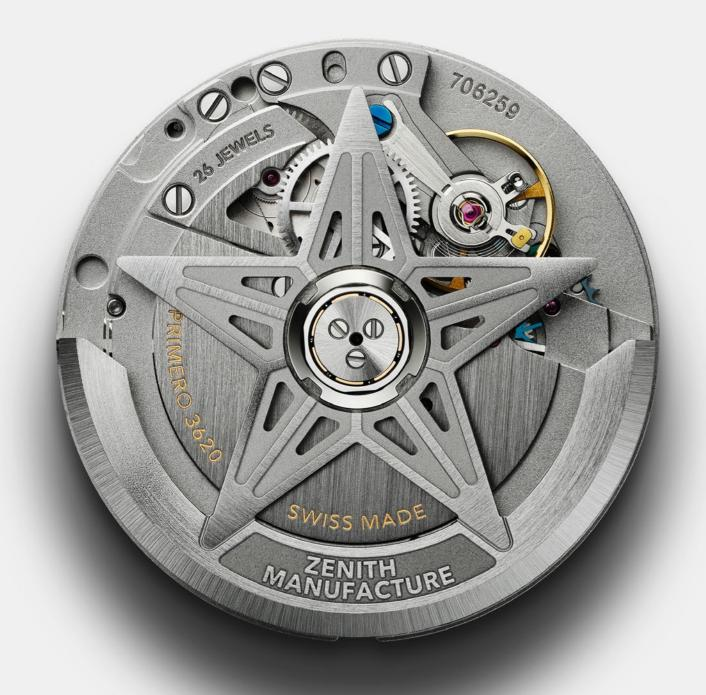
his exceptional performance is delivered by the new El Primero 3620. Built with a similar architecture as the El Primero 3600 1/10th of a second chronograph, this automatic manufacture movement visible through the sapphire display back drives the 1/10th of a second hand directly from the escapement, which beats at 5Hz (36'000 VpH), thus making it a "natural" fraction-of-asecond indication.
